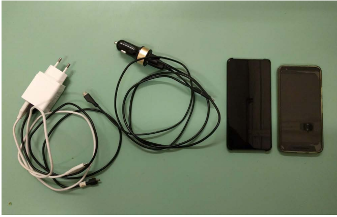
Double chargers for smartphone devices, both household plug and car battery, each with mini-USB and Type-C adapters.
